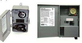
Optional UL Approved Control Panel complete with Class A Human Rated GFCI Protection, 24 Hour Mechanical Timer, and Photo Eye for Optional Light Kit. NEMA Type 3R weatherproof enclosure.
