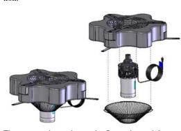
The motor unit attaches to the float using stainless steel hardware for a secure assembly. The 3 section, U.V. resistant, high density thermoplastic float allows for excellent durability with an attractive shape and low visibility. Rigid top and bottom screens help protect the unit from debris and reduce the likelihood of clogging.
